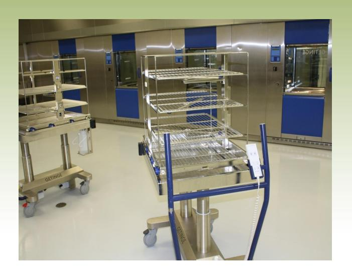
Use of height adjustable carts allows for proper body mechanics.
